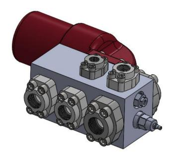
All in one manifold for the control of output oil from a subsea auxiliary or dirty work pack pump. Principally designed to reduce space in subsea hydraulic systems but also to increase reliability by eliminating a significant number of pipes and joints between components, reducing complexity, and simplifying maintenance.
